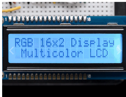
Figure 21: RGB backlight positive LCD Display
