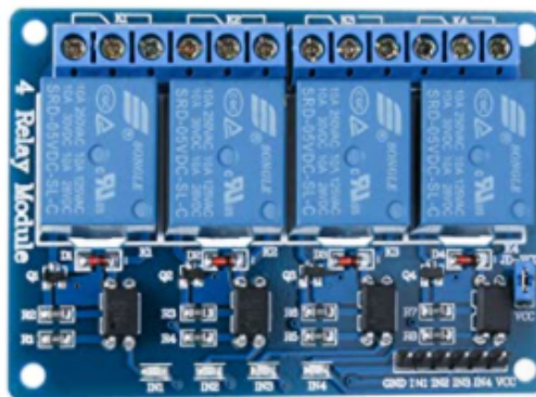
Figure 26. 4-Channel 5V Relay
